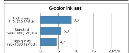
Print modes listed on this brochure are included in the printer's specifications. Profiles are created by selecting print modes according to the characteristics of each type of media. However, profiles are not prepared for all media types and print modes. If an appropriate profile is not provided, the profile can be created by using Mimaki Profile Master II.
