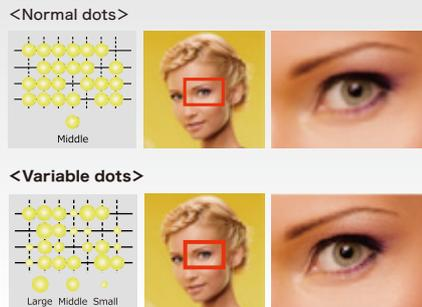
Dots are combined with the minimum size of 4pl to enable smooth color printing with less granular feeling.
