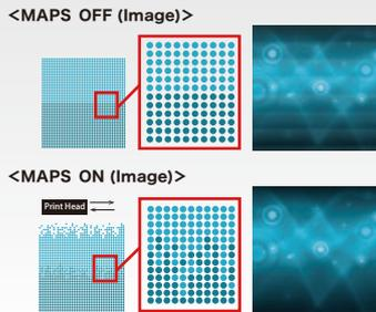
Based on printing conditions such as media/ink type and resolution, the most suitable gradation pattern is automatically selected and printed.
