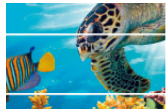
Gap/White streaks (Excessive feeding amount)
