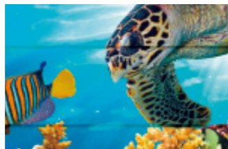
Overlap/Black streaks (Insufficient feeding amount)
