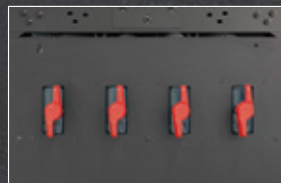
Vacuum zone valves
