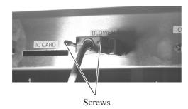
Insert one end of the signal wire cable for the blower into the connector of the electrical box.
