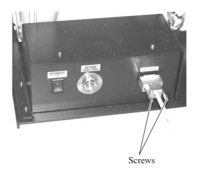
Insert the other end of the signal wire cable for the blower into the connector on the blower unit.
