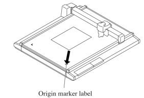
Place a sheet of A3 or larger paper in landscape orientation on the device while aligning the lower left corner of the paper to the origin marker label.
