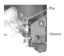
Insert the pin of head B into the tangential cutter while fitting the pin in the groove on the cutter.
