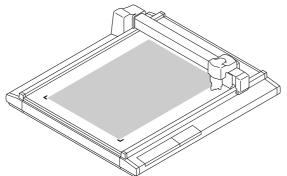
Place a work on the cutting panel.
