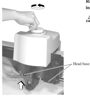
Raise the head using the height adjusting knob.
