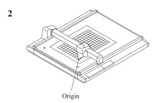
Establish an origin at the leftmost one of the ruled lines printed on the work. See page 2.40.
