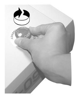
Turn the EMERGENCY button clockwise for unlocking.
