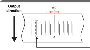
The dots at the fourth position counted from the zero position in the positive direction form a straight line. In this case, the dot position correction value is 4.0.
