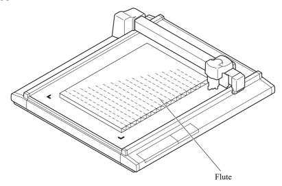
Place the corrugated board in such a way that its flutes are in parallel to the Y-axis of this device. To set a marking pressure in terms of the Y-axis direction, specify how far the pressure is reduced from the pressure value designated in the [CUTTING CONDITIONS]. ( P. 2-23)
