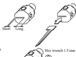
2. Using the supplied hex wrench (1.5mm), fix the blade by tightening the fixing screw.
