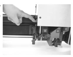
4. Tight the both fixing screws on the head alternately.
