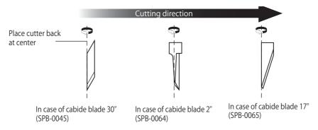
In pattern B, the tool is installed with tilted. Pattern B has to be adjusted so that horizontal lines and vertical lines are arranged in a straight line respectively along X- and Y-axes.
