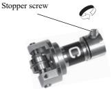
2. Insert the pin of unit C into the marking roller while fitting the pin in the groove on the roller.
