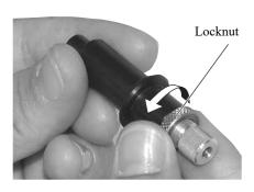
2. Turning the adjusting knob counterclockwise, draw out the holder B from the holder A.
