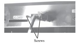
2. Insert the other end of the signal wire cable for the blower into the connector on the blower unit (option).
