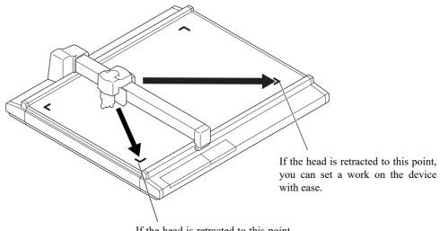
If the head is retracted to this point, you can set a tool with ease.
