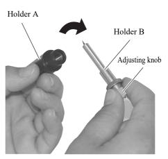
3. Replace the blade tip with a new one using a pair of tweezers.
