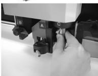
3. Tighten the stopper screw with the screwdriver supplied with the device as an accessory.
