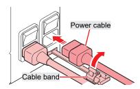
5 Plug the power plug into the power outlet.
