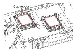
5 Check to confirm that the cap slider is not tilted once cleaning is complete.
