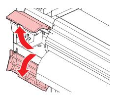
**2** Remove the side screw, and detach the media holder stopper.
