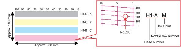
6 Select the "head number and nozzle row" for nozzle recovery, then press the [ENTER] key.
