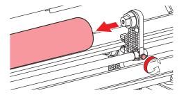
Tighten the retaining screw on the rear right roll holder.
