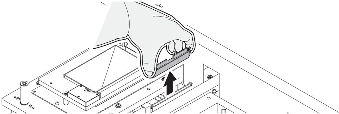
5 Remove the ink from the wiper, bracket and the vicinity of the wiper insertion hole using a cotton swab dampened with the cleaning solution.
