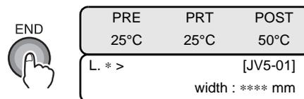
The display shown below will be kept until the temperatures of all the heaters reach their respective preset levels. When the temperatures of all the heaters have reached their respective preset levels, the buzzer sounds and the CONSTANT lamps for the Pre-heater, Print heater and Post-heater light up. Then the printer enters REMOTE mode.
