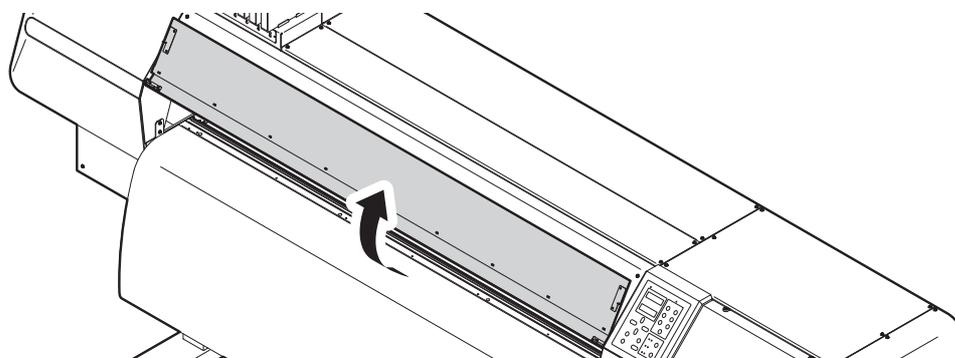
**4 Loosen the screw securing the cutter unit and remove the cutter unit.**
