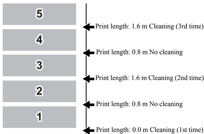
When five copies of an image 80 cm long are printed in series, cleaning is repeated before printing each of the 1st, 3rd, and 5th copies.
