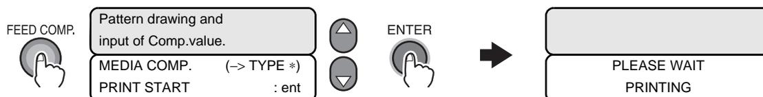
3 By judging from the output pattern, enter a correction value using the [ $\blacktriangle$ ] or [ $\blacktriangledown$ ] key.
