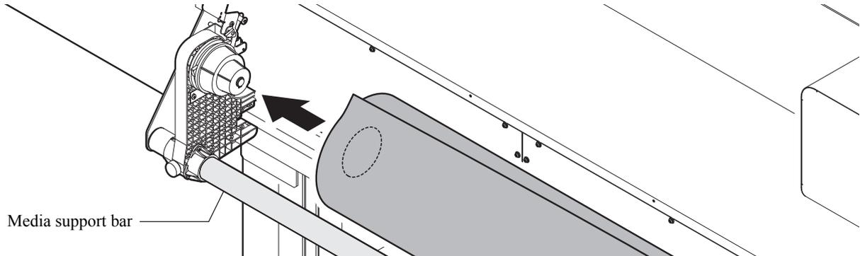
**4 Loosen the screw for the right roll holder, and insert the right roll holder into the core of the roll media.**
