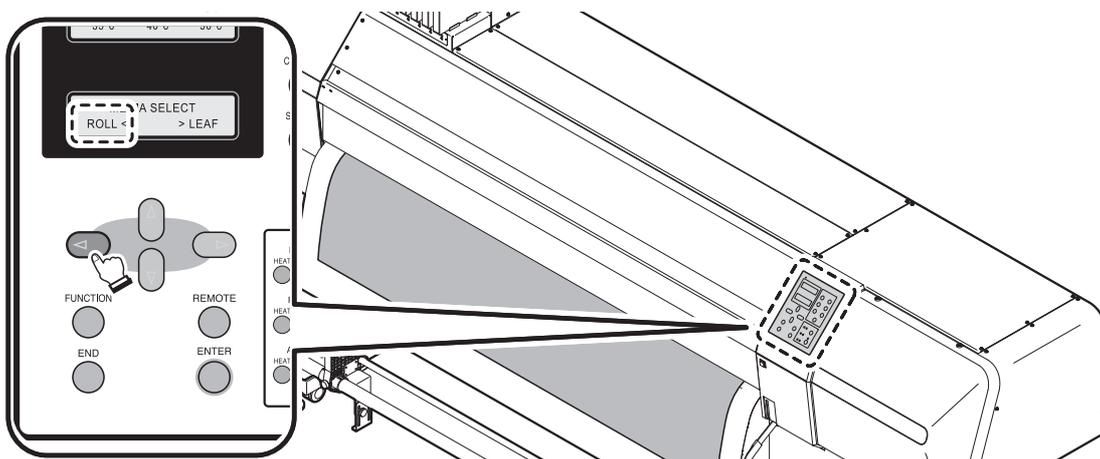
**16 Press the Jog key [▼] to feed the media up to the paper tube of the take-up device.**
