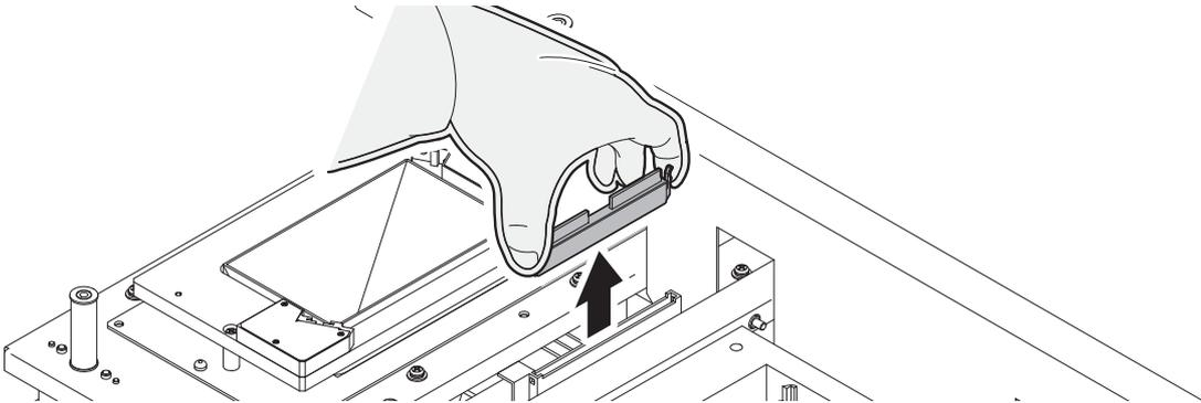
5 Remove the ink from the wiper and the bracket using a cotton swab dampened with the cleaning solution.
