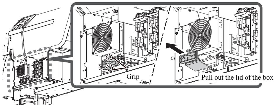
5 Remove the stains stuck on the lid of the box and fix it as originally.
