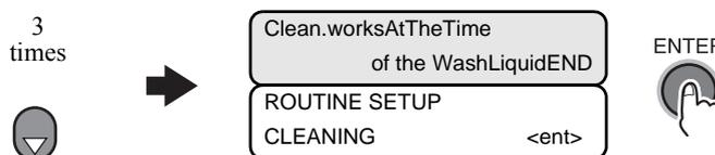
4 Select the interval at which cleaning is to be performed periodically, using the [ $\blacktriangle$ ] or [ $\blacktriangledown$ ] key.
