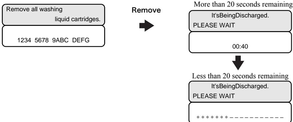
**7 When the display shown below appears, set the cleaning liquid cartridge in the ink station.**
