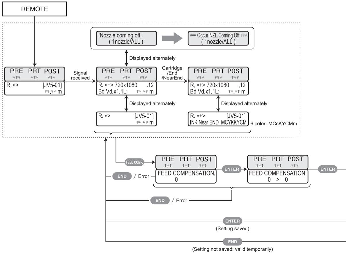
Pressing HEATER key or ENTER key in operations below is to be performed when the printer is in any state shown within the chart enclosed with dotted line above.
