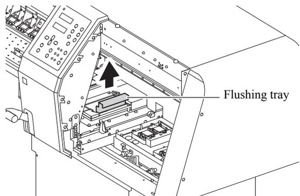
4 Fix the flushing tray. Also, fix the F-BOX filter and F-BOX filter base in the same manner.
