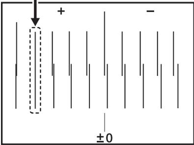
The dots at the fourth position counted from the zero position in the positive direction form a straight line. In this case, the dot position correction value is 4.0.
