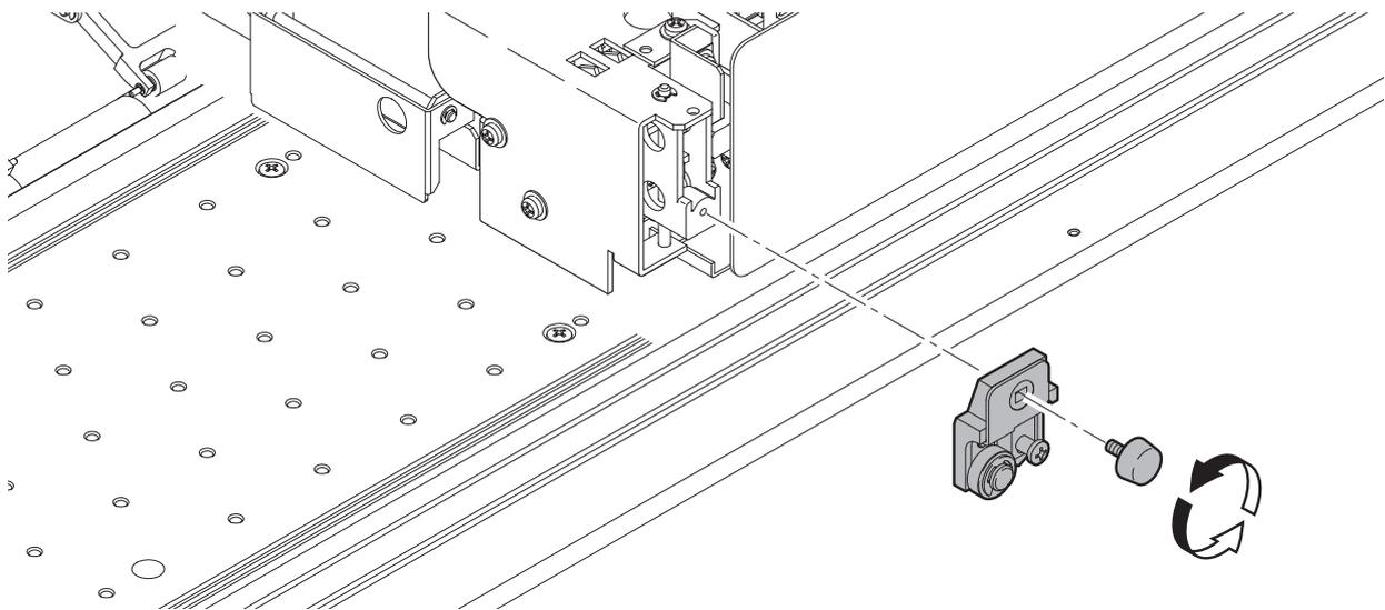
**5 Remove the roller, and install it on the new cutter blade holder assembly.**
