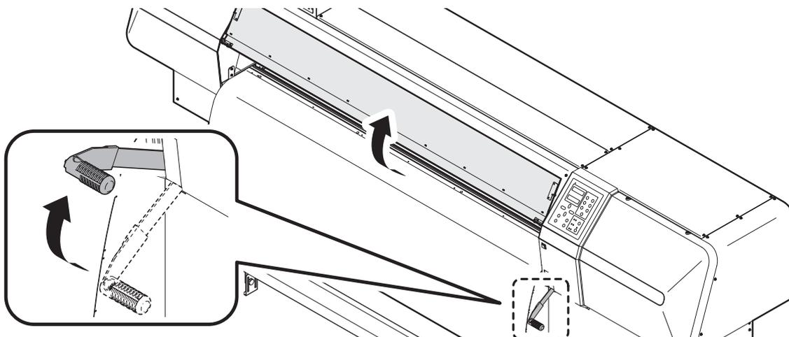
9 Pull out the roll media gently and then stop pulling when locked lightly.
