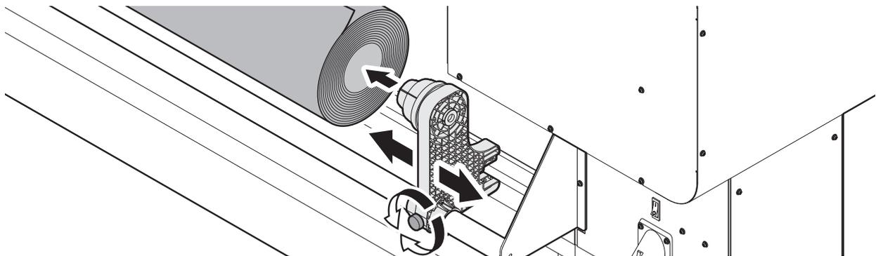
**5 At the rear of the printer, unroll the roll media by such a length that the unrolled part is long enough to reach the front end of the platen.**
