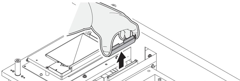
6 Remove the ink from the wiper and the bracket using a cotton swab dampened with the cleaning solution.
