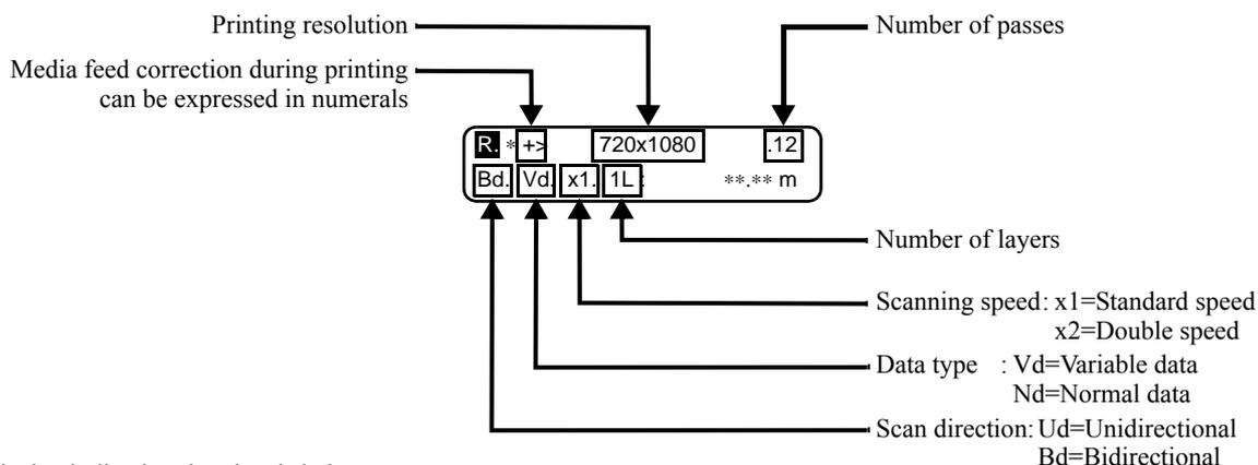
The display indicating that data is being received is alternated with the normal display.
