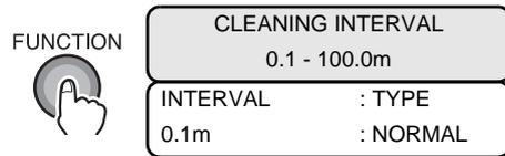
5 At this point, either of [CLEANING INTERVAL] and [CLEANING TYPE] can be selected by pressing the [◀] or [▶] key.
