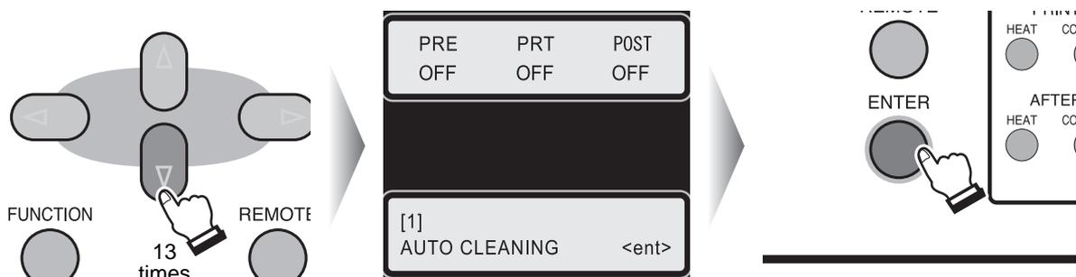
4 Press the [▲] or [▼] key to set ON/OFF of automatic cleaning.
