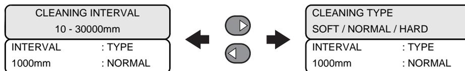
6 Set the value of [CLEANING INTERVAL] using the [▲] or [▼] key. Change the display by pressing the [◀] or [▶] key, select a type on the [CLEANING TYPE] display using the [▲] or [▼] key, and press the [ENTER] key.
