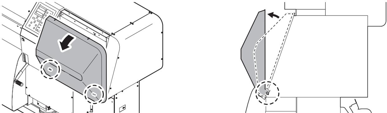
**3** Pull out the maintenance cover upward.
