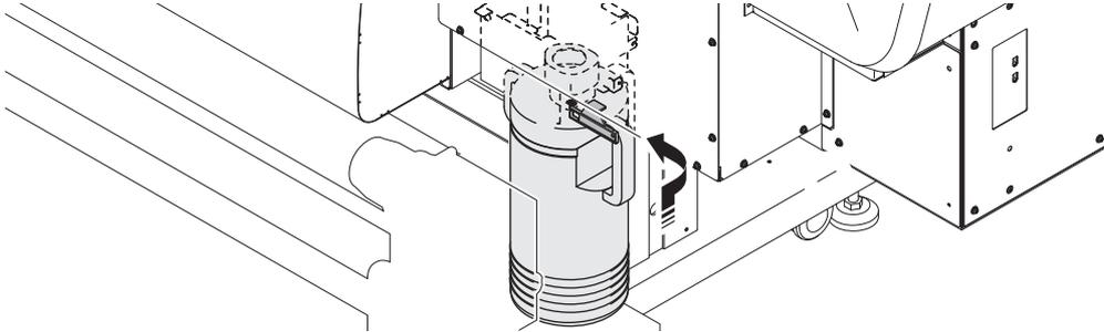
**6** Close the waste ink tank guard, and secure it with the screw so that the waste ink tank is secured.
