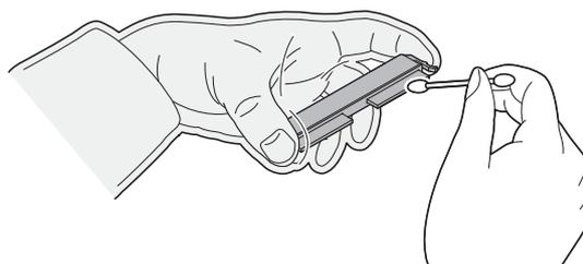
7 After cleaning the wiper, install it in position by holding the projections at both ends. Be careful of the direction of the wiper.
