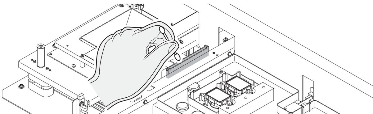
**5 Install the wiper by holding the projections at both ends.**
