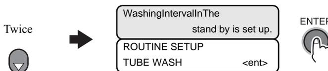
**4** Input the interval at which cleaning operation is to be performed periodically, using the [▲] or [▼] key.
