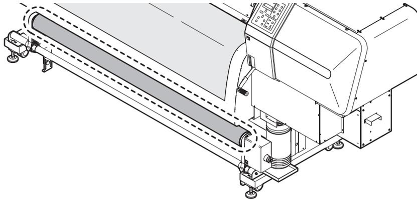
13 Adjust the level adjusters of the take-up device so that the bottom of each of them rests on the floor and secure them by tightening the thumb screws.
