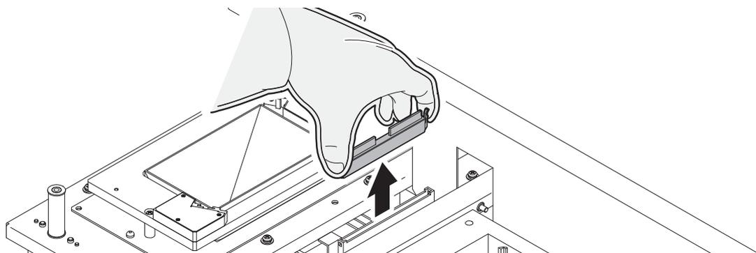
**4 Clean the wiper guide shaft using a cotton swab or cloth.**
