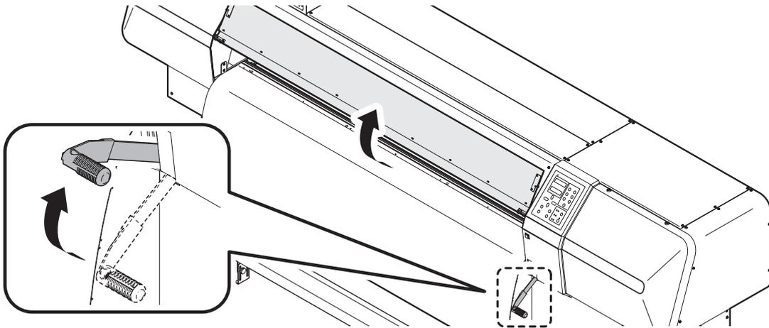
2 Insert the cut sheet media between the platen and the pinch rollers.
