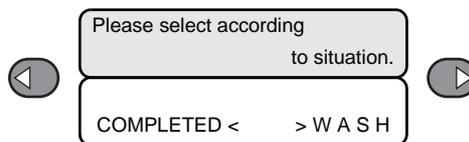
**10 Press the [◀] key when this function is to be terminated without discharging the cleaning solution.**
