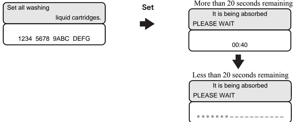
**8 When the display shown below appears, remove the cleaning liquid cartridge from the ink station.**
