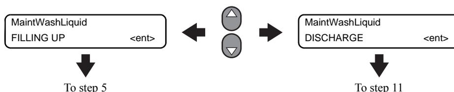
**5 Press the [ENTER] key to go to the lower level of hierarchy and supply the cleaning solution.**
