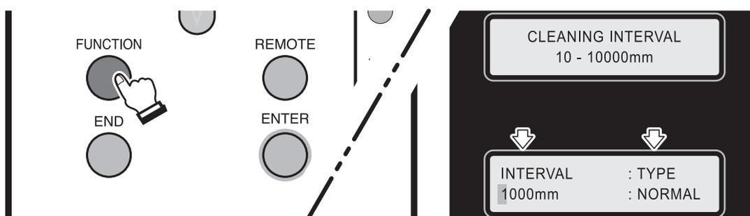
6 Press the [FUNCTION] key to go to the lower level of hierarchy and press the [▲] or [▼] key to input [CLEANING TYPE].
