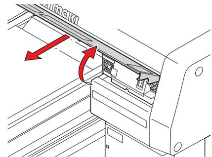
**6** Dip washing liquid into the cleaning swab, and wipe dirt of the wiper nozzle.
