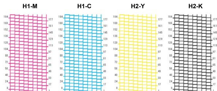
**5** Select the Nozzle line that needs **NOZZLE RECOVERY** by pressing **▲** **▲** key. Then press **ENTER** key.
